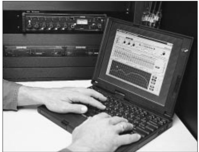
Example of a PC-controlled feedback reducer and equalizer. (Two Shure DFR11EQs shown on bottom of rack.)
