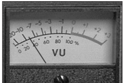
Average reading if level is set too low; may result in inadequate signal.
