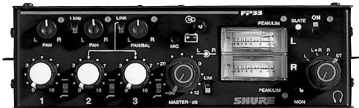
Example of a microphone mixer (Shure FP33 shown).
